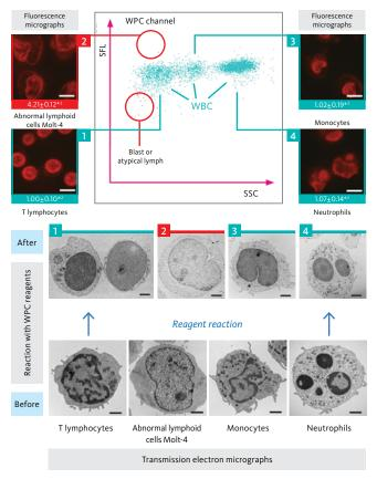
\*2 Image analysis was performed and the fluorescence intensity (mean±SD) of each white blood cell subtype was expressed, taking the mean fluorescence intensity of T lymphocytes as 1.0.
